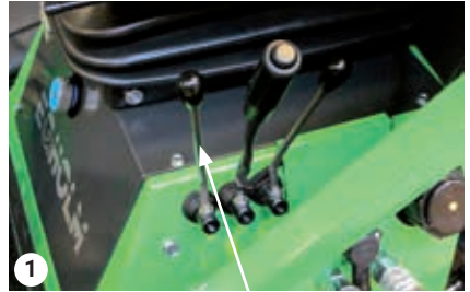
The snow v-blade is raised using lever A
