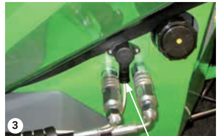
Fit the hydraulic hoses and power plug
