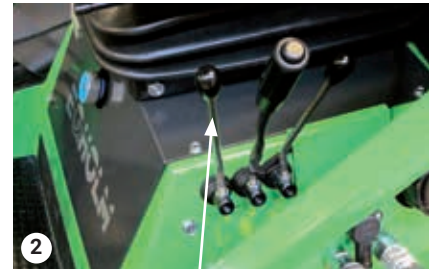
Use lever A to lower the snow v-blade
