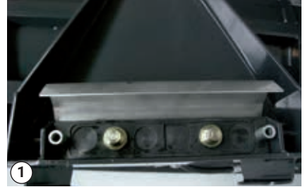
Cleaning the couplings
