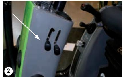
Transport lock in unlocked position
