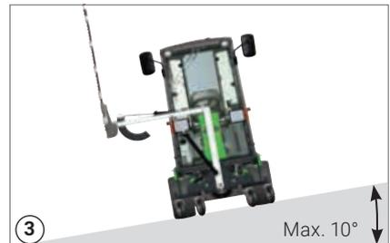
Do not drive on slopes with an incline of more than 10°
